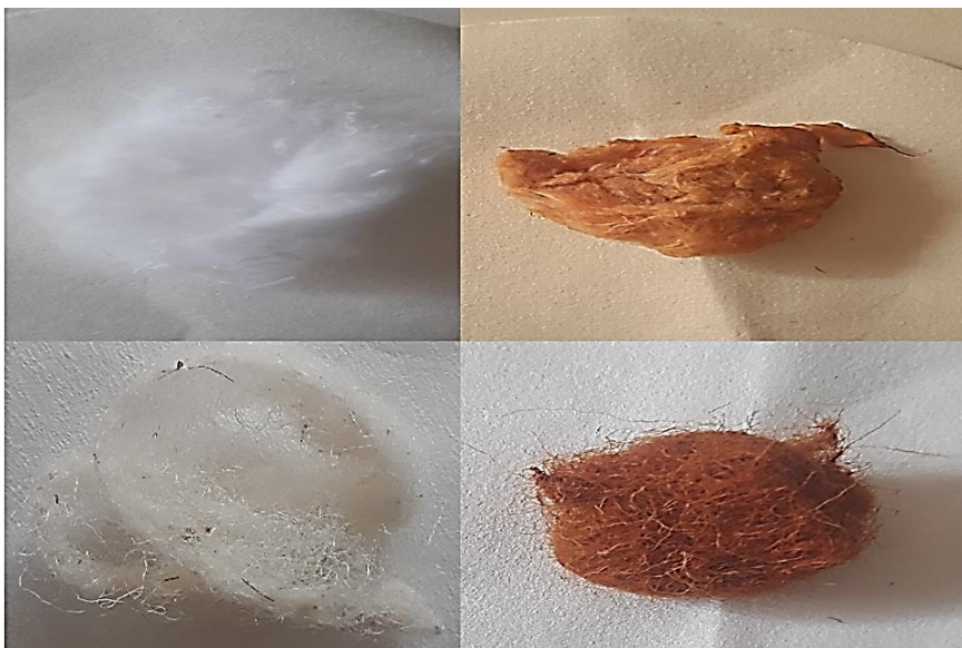
Fig.12: Visual appearance of cotton and wool fabrics before (left) and after (right) the dyeing process with the synthesized Mannich base derivative. The distinct shades of orange and reddish-brown confirm the successful fixation and chemical affinity of the dye under the specified pH conditions (pH 9 for cotton and pH 4 for wool).
