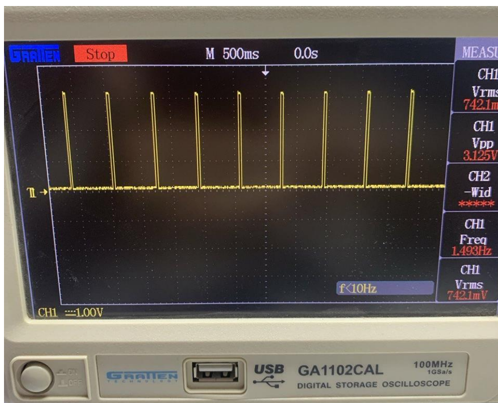
Fig. 8: The extracted pulses at the output of the comparator.
