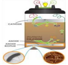
Mechanism of single chamber MFC- Anode and cathode separated by cathode specific membrane. Microbes at anode oxidize organic fuel generates electrons and protons. Protons move to the cathode compartment through the membrane.Electrons transferred to the cathode compartment through external circuit to generate current.Electrons and protons are consumed in cathode chamber, combining with O2 to form water.
